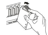
③ Secure the module with an additional screw (M3 x 12) to the base unit if large vibration is expected. This screw is not supplied with the module.
